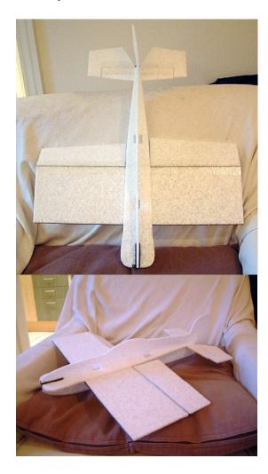
All parts made from 5mm EPP sheet
